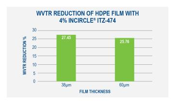
The performance improvement found with INCIRCLE® ITZ-474 has been validated in a variety of HDPE resins from several different resin producers. This new moisture barrier enhancement masterbatch provides film formulators with additional design possibilities in barrier films.
